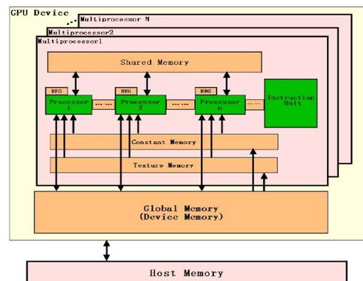
Fig.1 Device architecture of GPU.
