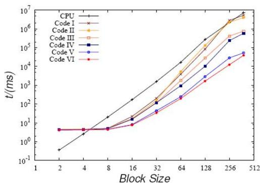
(a) Processing time of different codes and CPU versus *Block Size*.
