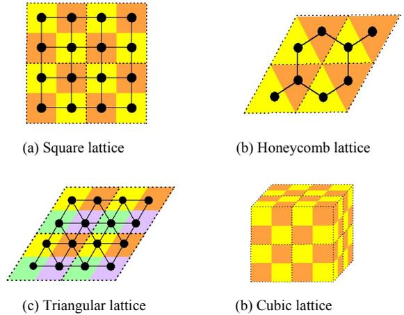
Fig. 2 Schematic visualization of the implementations of the Ising model on various lattices on GPU: the areas enclosed by dotted lines are subcells simulated in parallel. The spins in the boxes with the same color are operated in parallel.
