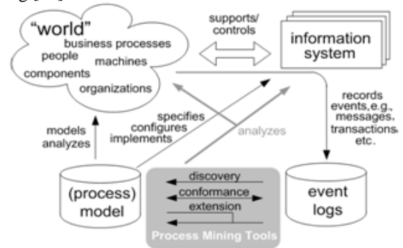
Fig. 1. Process mining overview and its types: (1) Discovery, (2) Conformance, and (3) Extension.
