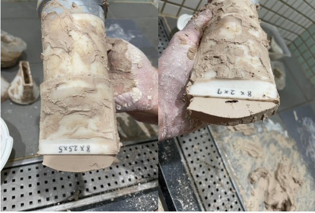
Fig. 21. Extrusion experiment (8×2.5×5) and (8×2×7).
