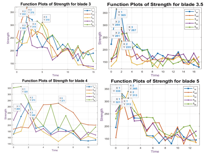
Fig. 15. Function plots of strength with different spacing of continuous helical blades.
